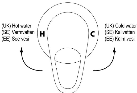
(UK) NOTE: For **shower cabins** without a thermostat, the flow controller adjusts both water flow and the water temperature. For **steam cabins**, the flow controller only adjusts the water flow. In this case the water temperature is adjusted by using the thermostat.
