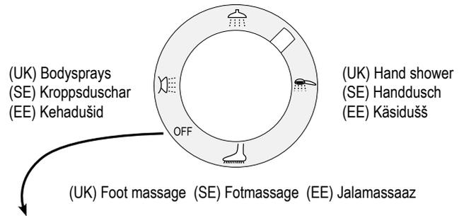
(UK) OFF (only on steam cabins): When you want to use the steam function, turn the handle to OFF mode to fill the steam water tank with water. **IMPORTANT!** When you will stop using the cabin, always turn off the water by using the flow controller and turn the divert to any other mode than OFF.
